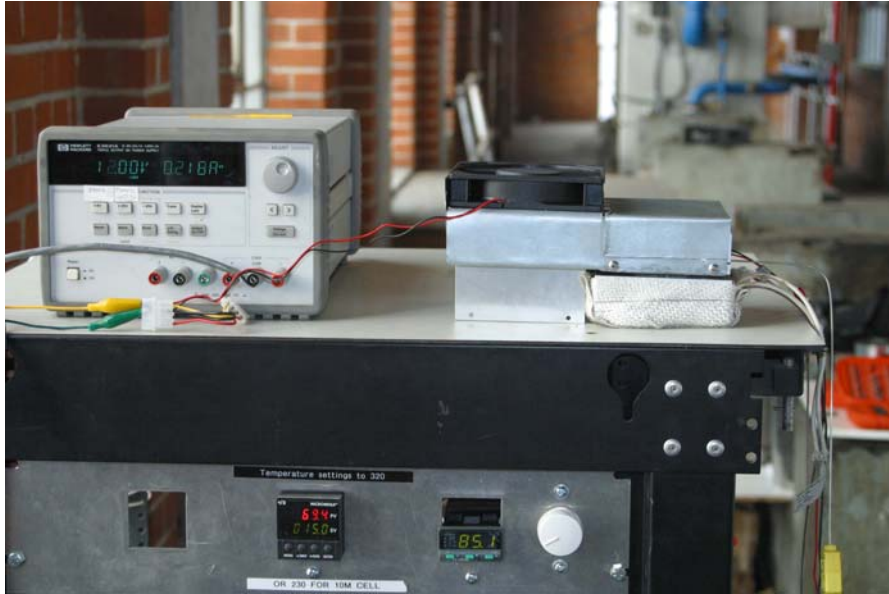
Figure 7: Bench testing the generator
