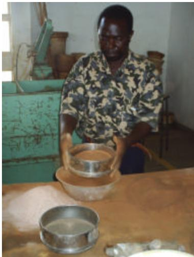
Working with Jameson Mujaye at the National Institute of Scientific Research (NISIR Ceramic Division) we made 5 test bricks, using different mixtures of local high magnesium red clay, mullite grog, and sawdust. These test bricks will be ready in October 2004.
