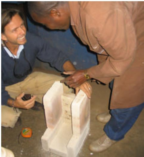
The key to producing a smokeless stove is to find inexpensive, local, and durable materials for the Rocket Stove combustion chamber. In Malawi, we have been blessed to work with Dedza Pottery. They have helped us produce a insulative refractory brick that is light (.67 g/cc) and durable.
