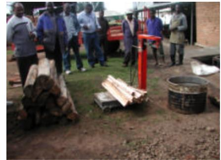
A visual comparison between the quantities of wood used (170kg) for the open fire vs. the amount of wood used (13kg) for the 100L Rocket stove. Independently tested by EP Lauderdale Tea Estates (Malawi)
