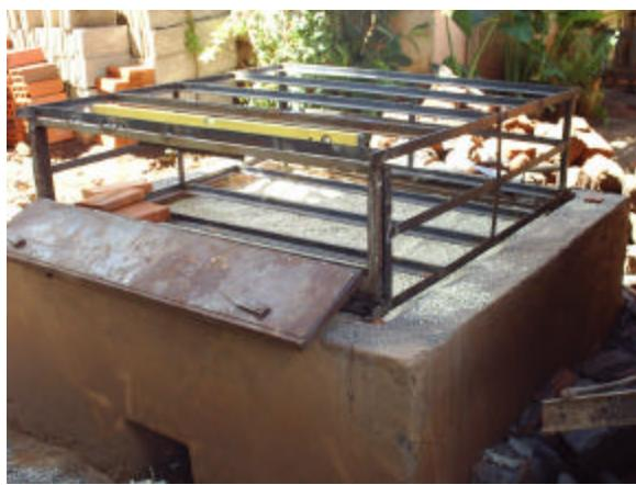
In March 2004, a new bread oven was designed that utilized a 5 mm T-Bar frame to directly support the clay baking tiles instead of the 2mm mild steel sheet metal baking compartment. The use of any metal in the baking compartment is an interim measure to assess if the general concept is acceptable to the bakers. The fourth prototype will not have an angle iron frame on the bottom of the baking compartment and will instead be supported entirely by clay bricks.
