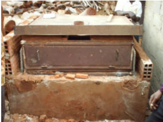
We then used a metal plate that was salvaged from the first prototype, to produce the interface between the stove and the chimney. Future models would not require the use of an entire metal plate.
