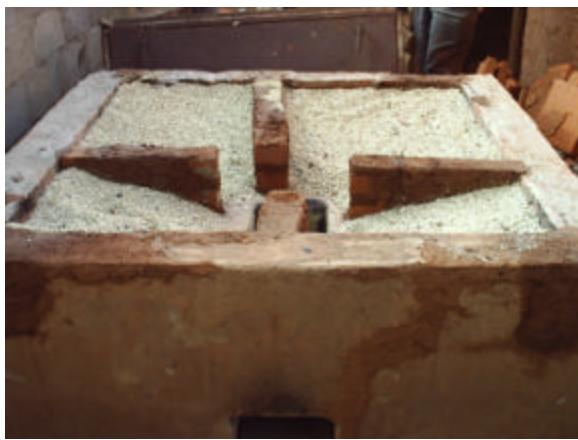
The third prototype was modified to incorporate 4 courses of bricks so as to offer more support to the baking compartment. The 4 corners of the outer structure were also reinforced with solid brick instead of thinner walled Ceramica Villa Pery building blocks.
