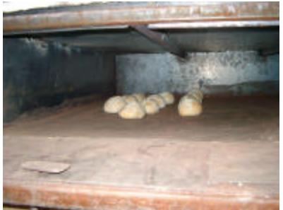
The rolls, which are cooked directly on clay tiles, require 300 degrees Celsius, as compared to 'loaf' type breads that require only 180 degrees Celsius. The 2mm sheet metal box (which has proved effective in Lesotho and Uganda) was not sturdy enough to withstand these higher temperatures. There were also other complaints such as uneven baking temperatures. The oven was too hot on the bottom and too cold on top.
