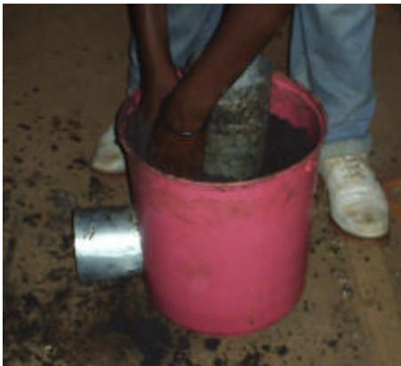
The bucket is then filled with clay sawdust. The mixture is tamped firmly into place.
