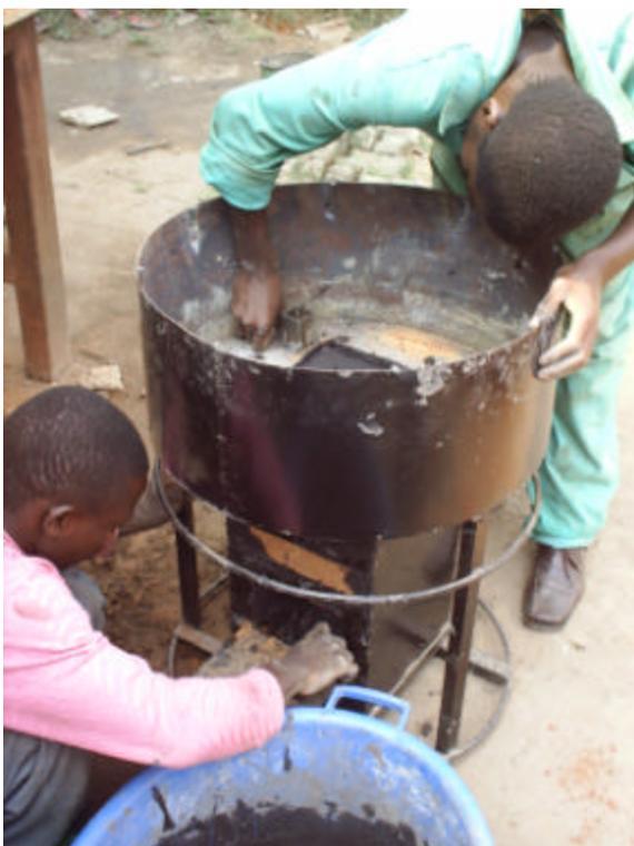
This Stove was originally produced for WFP and sent to Gondola. Unfortunately it was used before the mortar had dried which caused it to crack. When stove #3 was delivered, this stove was picked up and returned to Savepla on my last day in Mozambique. Instructions were left to retrofit the stove, Mark it with a #5 and then deliver it to ADPP on the 10<sup>th</sup> of September during Zana's first visit back to Chomoio.
