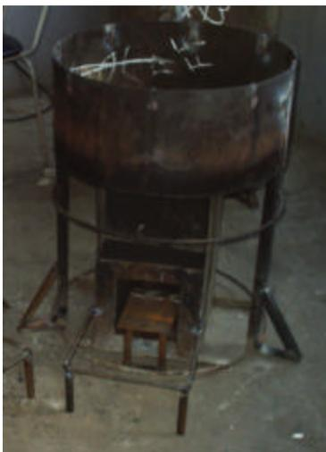
This stove is for Formigas del Futuro. It was built with lower grade clay/sawdust bricks. The liner bricks (with the exception of the two entrance bricks - 'E' on the left and 'C' on the right) were made with common brick clay last year. Although I am skeptical about the durability of these bricks, I thought it would be helpful to make one test stove using these lower quality bricks. If these bricks are successful, than it will greatly simplify production.
