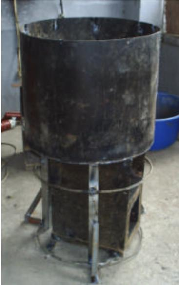
Savepla originally produced this stove as part of the three stoves purchased by ADPP. Unfortunately the stove diameter was too small to fit ADPP's pots. The stove sat unused for three months until I came back. The stove was picked up on Aug 20<sup>th</sup> . and retrofitted with ceramic bricks.. This stove is designed for the taller aluminum 80 L pots that ADPP and WFP both use.
