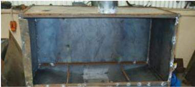
The upper part of the bread oven shell should be constructed with 1.6 mm.
