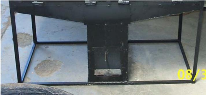
A sliding guillotine door on rails is attached above the fuel magazine/feed chamber. This door is used to reduce airflow after the oven has reached baking temperature.
