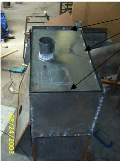
Coarse Vermiculite Insulation is placed around and on top of the bread oven annulus.
