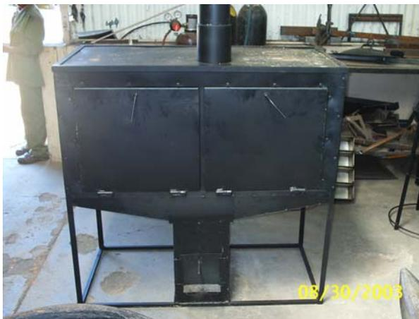
The detachable face plate (which allows for easy removal, maintenance, and repair of the baking compartment) is attached. Hinges are welded on to the insulated doors, and the stove is painted
