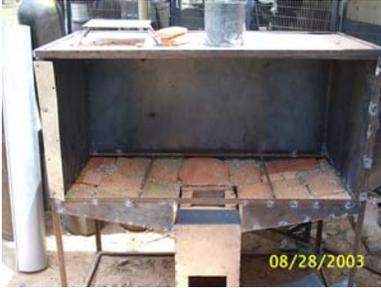
This thinner metal can be used because it will be covered with the insulative cement vermiculite mixture. Pictured here is the fired clay/vermiculite brick, which will be replaced with the cement vermiculite mixture in future models.
