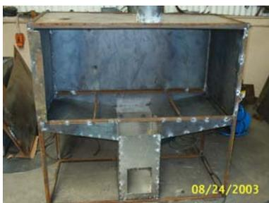
This is the outer shell and the combustion chamber of the bread oven.
