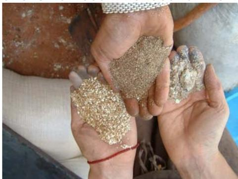
The above photo shows three different kinds of mica. Starting at bottom left and moving clockwise the picture shows medium or coarse vermiculite, fine vermiculite and finally unprocessed mica.
