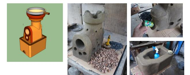
The Holey Roket Stove with a char box as drawn and as built and now drying. Notice the pusher rod (center photo) and the char pocket (upper right photo) on which a can of sardines may fit at the cover and the char box (lower right). Another possible plug would be plaster of paris but should be built only after the stove was fired in the kiln to ensure a tight fit. .
