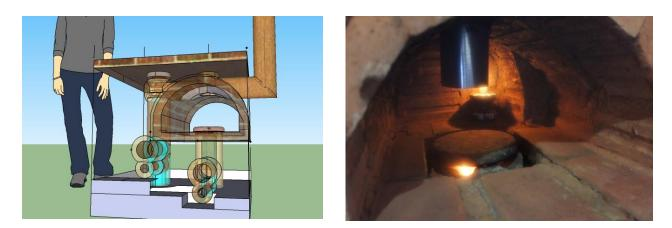
The oven chamber features the holey roket stove beneath the oven floor, a clay disc to deflect the hot gases sideways and unto the walls of the oven, an extended metal cylinder at the chimney. The combination of the two deflectors (the disc and the cylinder) causes the heat to circulate inside the chamber thus give a more uniform and retained heat. My thanks go to Jon and Flip Anderson and Larry Winiarski for the lessons I gathered from their earth oven stove.
