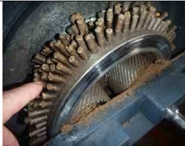
Ring-die press from AgriconSA in action (Photo Christa Roth)
