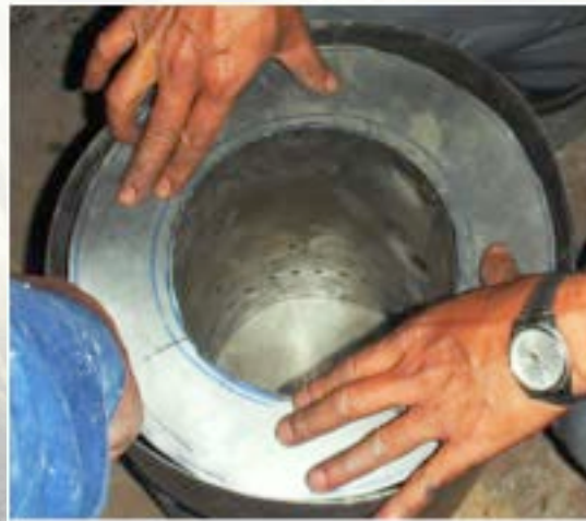
Top of pyrolysis chamber
