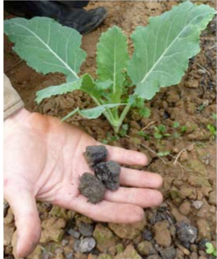
Biochar from open fire (produced possibly around 500-550C – temperature measurement taken in the char/ash layer of the open fire)
