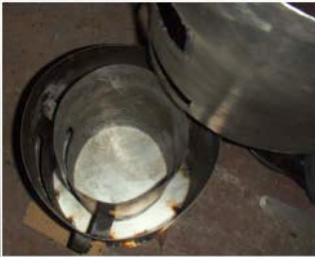
Lugs to position pyrolysis chamber
