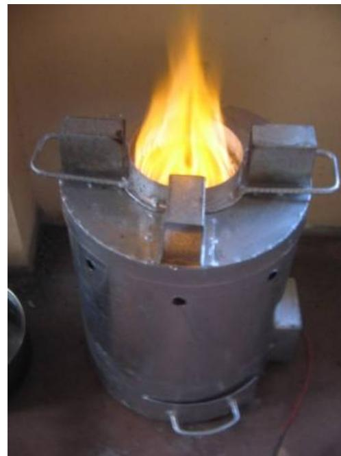
during operation. Beneath the inner cylinder is a grate that holds the fuel while being gasified. Small computer 12-DC fan is used to supply the air needed for gasification. The cover, where the four support stands is in place, holds the pot during cooking. The plate-type burner burns the gas emitted from the reactor. It is designed to be removable to allow easy reloading of pellets for continuous operation.
