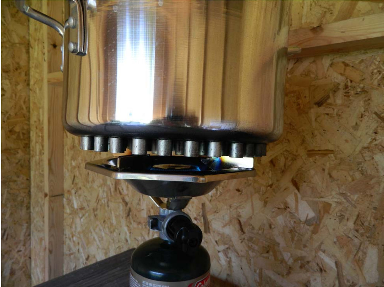
Figure 1: The propane stove with the finned pot. The bottom of the pot was painted black before testing, to give equal radiative heat transfer as the regular pot.
