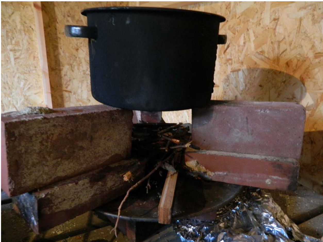
Figure 2: Open fire setup with the regular pot. The distance from the bottom of the pot to the base of the system was 6 inches (15 cm).
