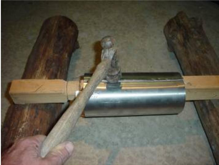
The folded edges of the riser component are interlocked and pounded into a closed seam with a ball peen hammer.
