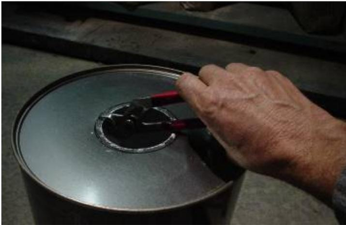
Using a very square-ended pliers (like a channel lock), carefully fold down the metal (approximately 10 degrees) precisely at the outer circle. This causes the metal to bend exactly along that line when struck with a ball-peen hammer.
