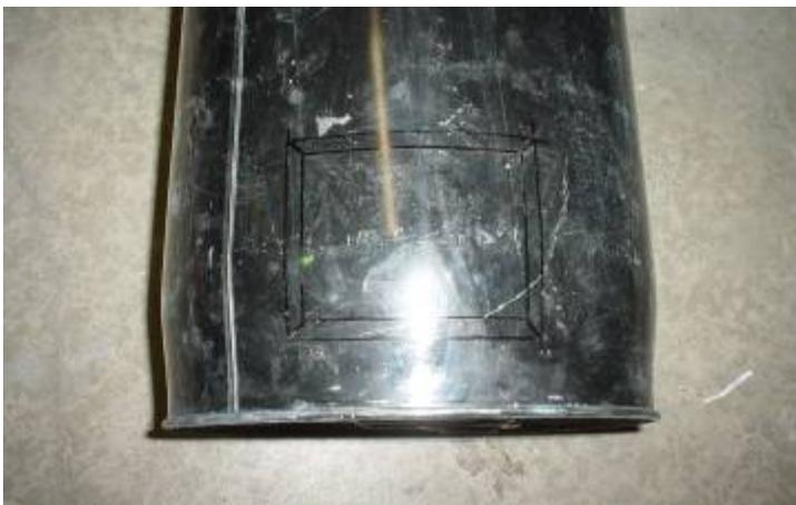
As with the opening on the top of the stove body, a second rectangle is drawn inside the fuel magazine placement mark. This second line will be the cut line.
