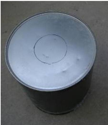
Using the now-formed riser tube as a template, trace the location of its future placement in the center of the can.
