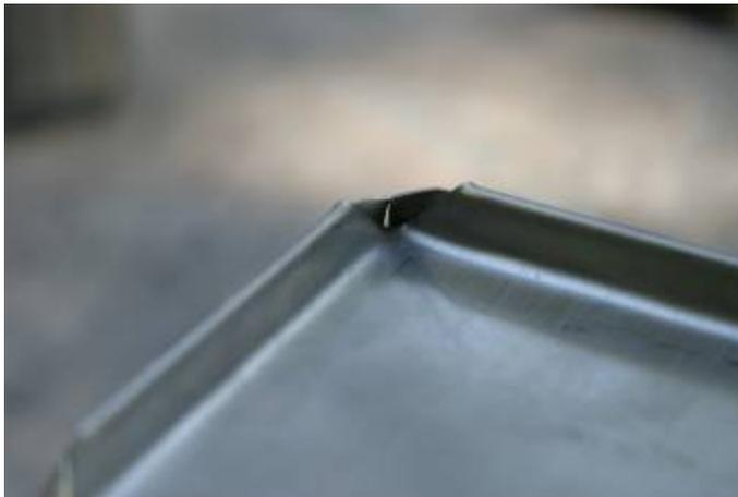
The corners of the fuel magazine are bent inward to retain the end cap. The resulting three-piece structure is quite rigid.
