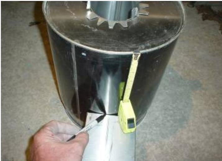
With this measurement, and using the fuel magazine as a template, trace the location of the magazine placement on the side of the can. The magazine should open on the opposite side of the can from the location of the spout-and-plug, on what is now the bottom of the stove body.
