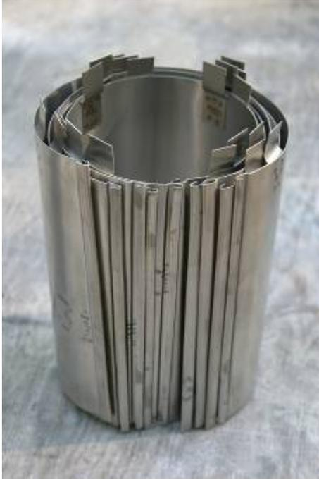
The 310 stainless components for the combustion chamber nest pretty well, making for more efficient packing and shipping. These are the riser pieces.
