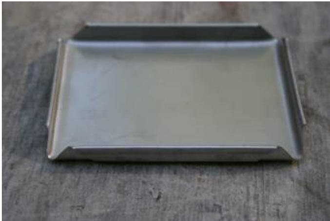
The end cap for the fuel magazine section of the combustion chamber.
