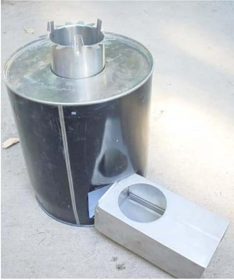
Lift the riser piece part-way out of its hole (so the fuel magazine can clear the tabs), and insert the fuel magazine into the side opening. Then, drop the riser onto the fuel magazine. Holding the two components tightly together, bend the fastening tabs (by hand) under the top edge of the fuel magazine to secure the structure.
