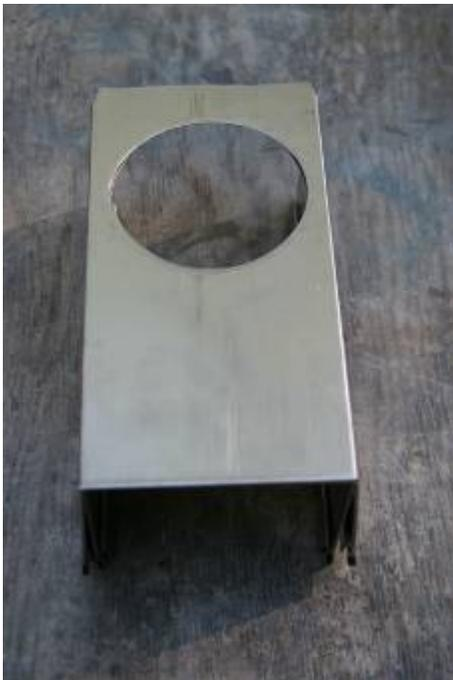
This is larger of the three pieces that make up the fuel magazine section of the combustion chamber.
