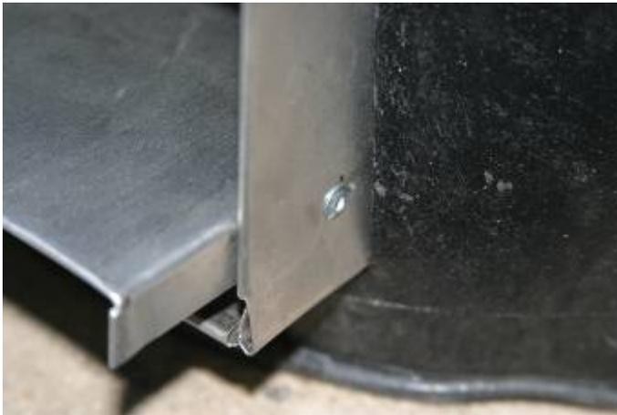
Fit the fuel feed shelf into the magazine, positioning it so that the inner edge aligns with the circumference perimeter of the riser. Affix the shelf with pop-rivets on either side, as shown.
