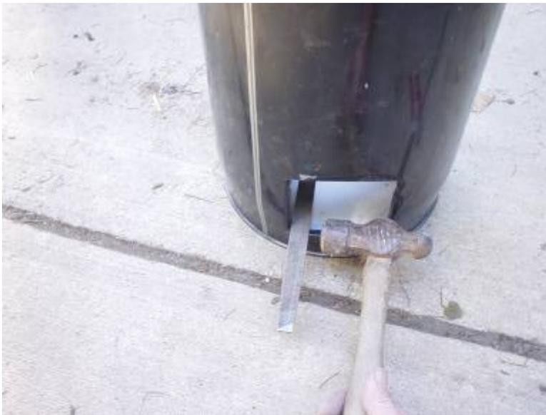
Since the hammer edge is round, but we need square corners to accommodate the fuel magazine, I used a hard, rectangular object to form them. For example, pound on the side of a heavy metal file set against the corner to square-up the bend.
