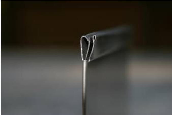
The edge of the larger piece of the fuel magazine is bent to accept the bottom piece.
