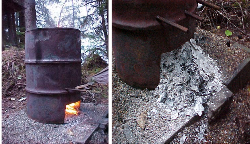
Figure 9: Burn barrel in Figure 8 burning paper, cardboard, and some plastic packaging material (no food waste, cans, or glass).
