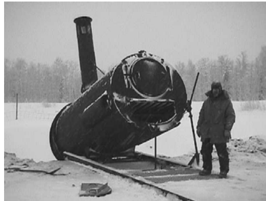
Figure A-8: Winter clean-out using Handy-Man jack.
