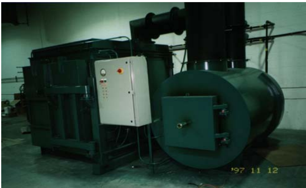
Figure 15: Thermal Oxidation System
