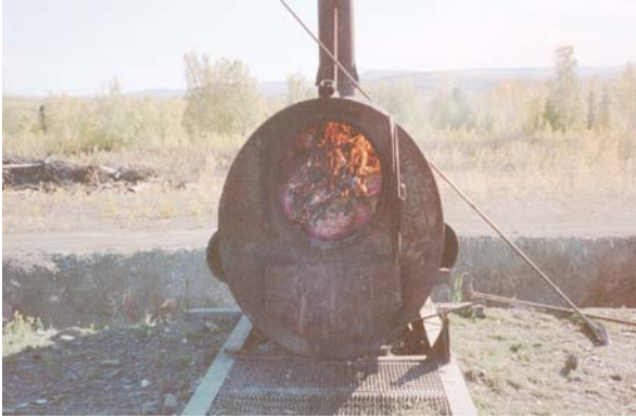
Figure A-3: Burn box after ignition.
