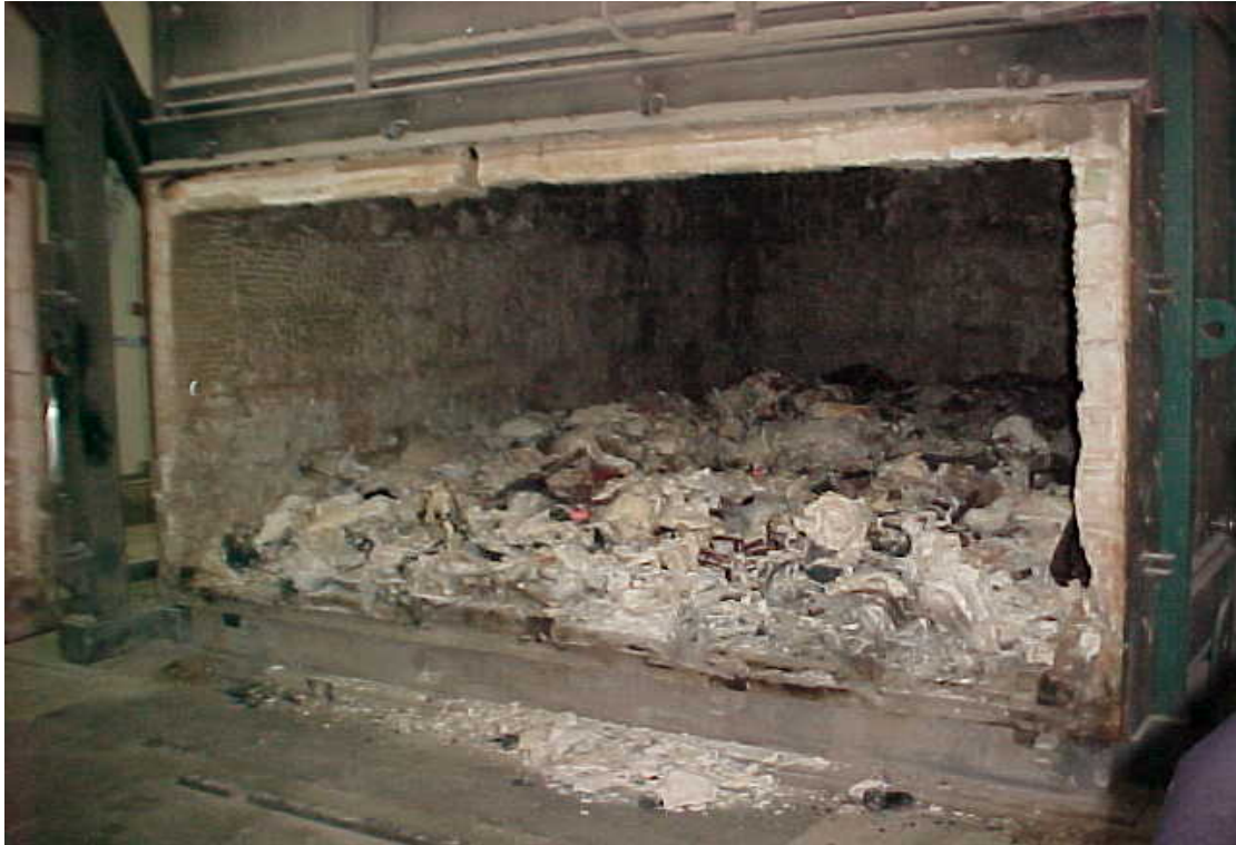
Figure 16: Thermal Oxidation System – Skagway, Alaska Primary Chamber Showing Ash After Burn-Down
