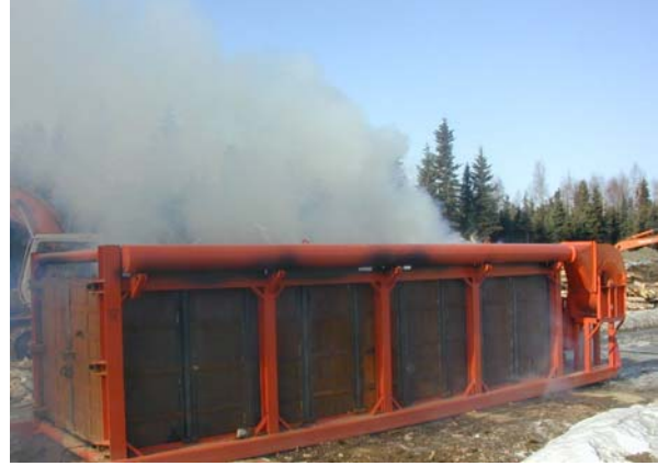
Figure 12: Horizontal above ground air curtain incinerator during start-up (note 100% opacity).
