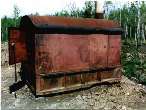
Side of Box. The box was made from a dump truck bed and steel plating. Note air intake vent near the front of the box.
