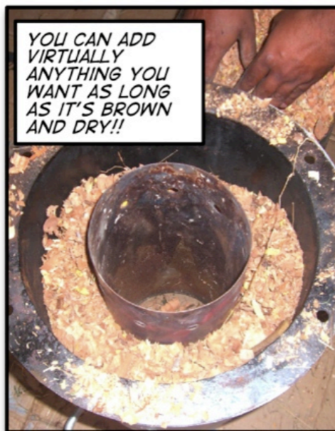
PACK THE BIO WASTE INTO THE GASSIFIER SPACE
