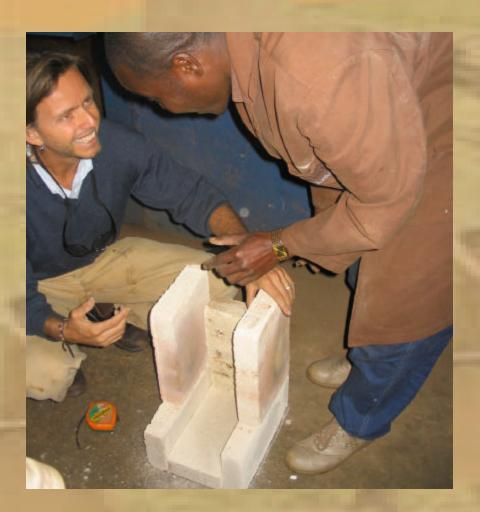
One of the keys to producing a smokeless Rocket stove is to find inexpensive, local, and durable materials for the combustion chamber. In Malawi, we have been blessed to work with Dedza Pottery. They have helped us produce an insulative refractory brick that is light (0.67 g/cc) and durable. The bricks are made with:
