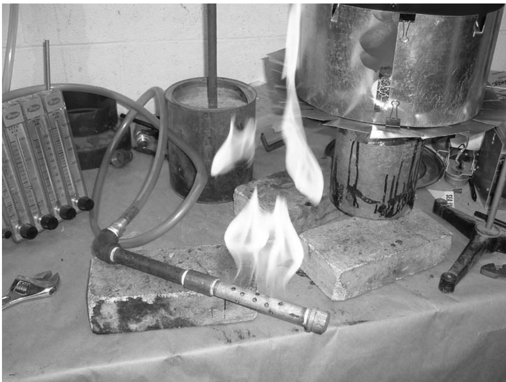
Figure 1.2: The burner in operation at about the middle power level. The flame in this photo has an unusually "tongued" appearance, partly caused by the camera flash.
