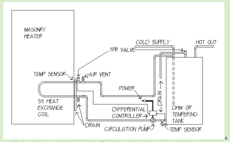
controller is required to sense when the heater is being fired or the water from the heater is warmer than the water in the tank.
