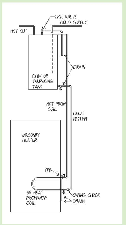
A thermosyphon system is the simplest. It requires that the storage tank be located higher than the coil. Best efficiency is obtained when horizontal distance to the tank is 4 ft. (1.2 m) or less and the vertical distance is 6 feet (1.8m) or more.
