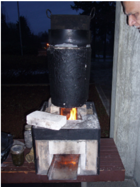
Figure 11: Weyer Dung-Burning Prototype Stove
