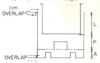
3. Stoves should have a total air inlet of at least half the area of the pot to wall channel gap. For the above stove 94 cm in circumference and with a gap of 6 mm this is 56 cm². A convenient size, then, is to have four airholes, about 3 cm by 4 cm each (A=3 cm) or 48 cm² in area, spaced symmetrically around the stove, but far enough away from the door and the seams to avoid weakening the wall. The airholes are cut
