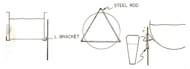
Pot supports should support the pot stably, yet be small in area so as not to shield the pot from the hot gases -- reducing heat transfer. Pot supports should not cause the stove wall to bend when heavily loaded as this can change the effective channel width and reduce performance.
