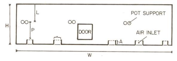
2. The template height H is determined by the sum of the airhole height A, the grate-to-pot height P (measured from the top of the grate), and the channel length L or, for spherical pots, the amount necessary to extend a few centimeters above the pot's maximum circumference. For cylindrical pots, L is determined by the desired channel length (chapter III)
