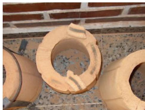
The center of some of the bricks did not fire high enough
