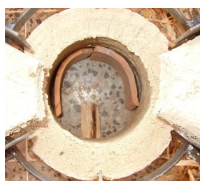
Thin roofing tiles fit nicely in the back of the combustion chamber to protect from stick abrasion
