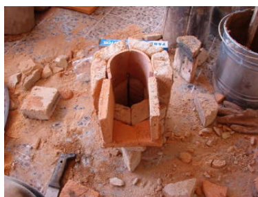
Upside down view of six brick stove shows how roofing tiles and baldosa can be used to protect from stick abrasion
