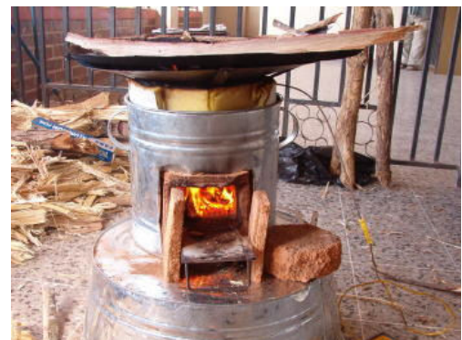
Testing six brick stove with comal and comal skirt
