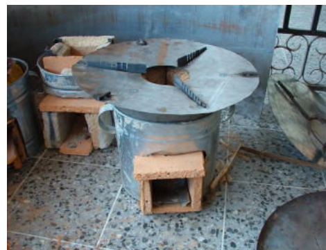
Comal shirt which built in pot supports and notches for adjustable skirt
