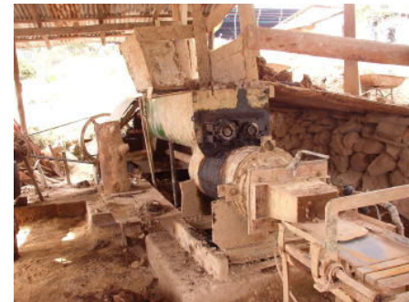
Combination mixer/extruder at the brickyard of Don Pedro is a dream come true for mass production of insulative bricks
