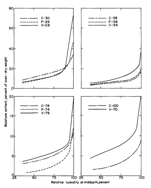
Fig. A-1. Moisture content-relative humidity relationships for 3½-in.-thick slabs of lightweight insulating concrete.
