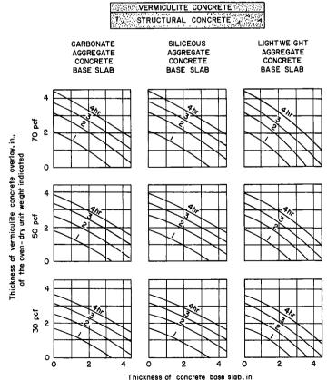
Fig. C-3. Fire endurance of slabs consisting of vermiculite concrete overlays on structural concrete base slabs.
