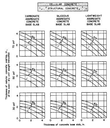
Fig. C-1. Fire endurance of slabs consisting of cellular concrete overlays on structural concrete base slabs.
