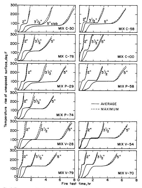
Fig. 2. Temperature rise of unexposed surface during fire tests.
