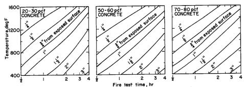
Fig. 5. Temperatures within insulating concrete slabs of different unit weights during fire tests.
