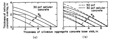
Fig. 6. Example of a design chart modified for a different overlay.
