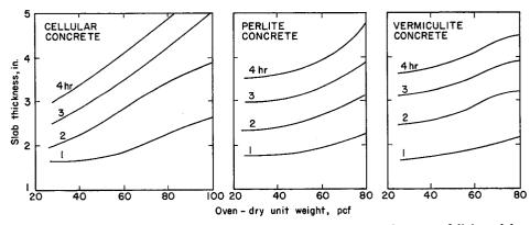
Fig. 4. Influence of unit weight and slab thickness on fire endurance of lightweight insulating concretes.
