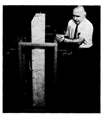
Fig. 1. Measuring the thickness of a 3x3-ft slab specimen.
