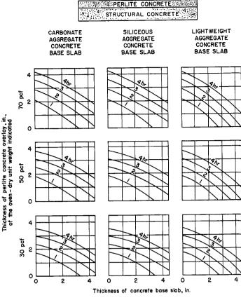
Fig. C-2. Fire endurance of slabs consisting of perlite concrete overlays on structural concrete base slabs.
