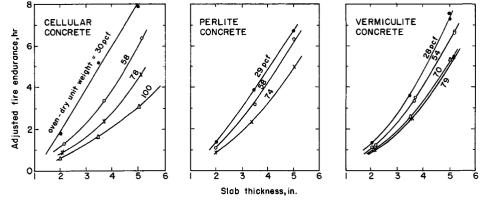
Fig. 3. Relationship between slab thickness and adjusted fire endurance for each of the concrete mixes.
