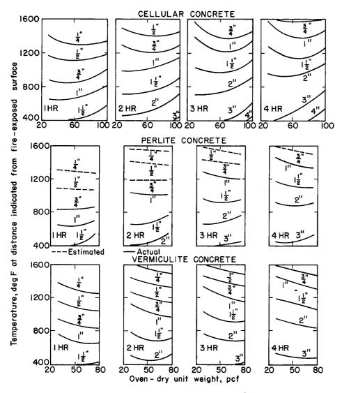
Fig. B-1. Temperatures within insulating concrete slabs during fire tests.
