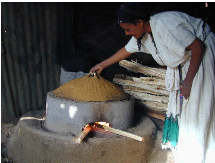
Baking Injera on the Mirt Stove
