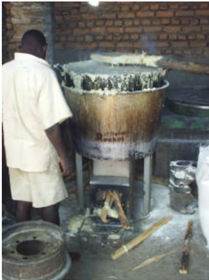
The Prison should be encouraged to use a single standardized pot. Having different size pots means that sometimes a large pot is placed in a small stove (or vice versa) which lowers efficiency and can damage the stove.
