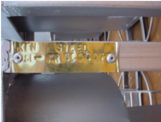
3. A numbered serial plate is attached to each stove. This allows ProBEC to track the stove in the future (who made the stove and when) and establishes the authenticity of the product for the purchaser.
