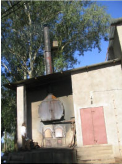
The second barn (shown left) uses a single combustion chamber (about half the size of the previous barn) that heats a 4500L kettle to 70C. This hot water is then piped through a radiator. A fan blows across the radiator and sends the hot air through 5 curing rooms. These barns are considerably more efficient (and expensive) than the traditional barn.
