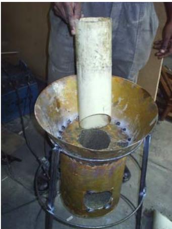
Make slurry of one part cement to 3 parts water. Use this slurry to thinly coat the inside of the entire combustion chamber.
