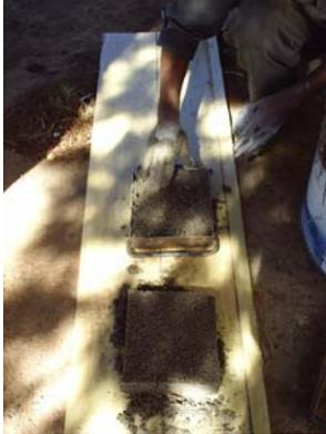
The three #25 stoves that were placed with WFP were made with fired VIC brick combustion chambers. These bricks are durable but they have a number of drawbacks. . They are expensive, heavy and complicated to produce. The new cement vermiculite bricks do not have these drawbacks but their durability still needs to be assessed. . The cement vermiculite bricks should be mortared together with the same mixture as the VIC bricks: a mixture of 1 part cement, 1 part cement and 1 part vermiculite.
