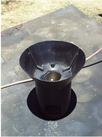
Then paint with red oxide. Allow to dry. Then coat with flat black enamel
