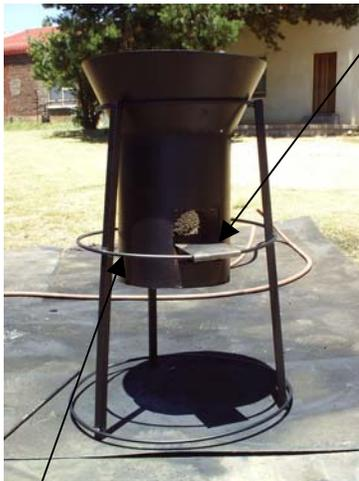
Shown here is the removable shelf that rests on the center ring. This design component will be changed in future models. Instead of having a removable shelf that spans from the combustion chamber to the support ring, the shelf will now be smaller and fixed to the combustion chamber. The shelf will be made from 3mm mild steel and will be similar in shape to the shelf in the Mozambican single pot stove. This design modification will decrease
