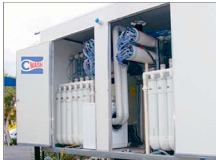
Cummins Corp's C-Wash system for treating and recycling waste water from commercial car wash operations
