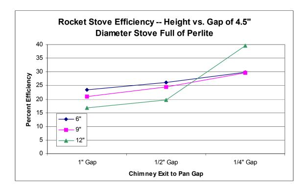
An important consideration, however, is that the <sup>1</sup>/<sub>4</sub>" gap sometimes caused the fire to burn out the top front of the feed magazine because not enough air was able to be drawn through the decreased gap to create the proper draft.
