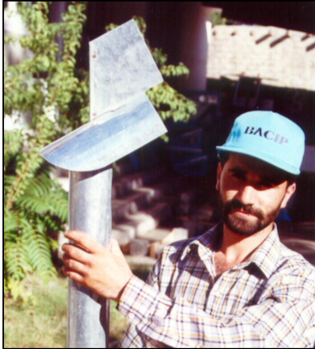
Low-cost chimney vane cap made of 26-gauge GI sheet metal, a pin and a bolt. Easily swivels around with every wind direction and avoids back-draft, especially on flat roofs.
