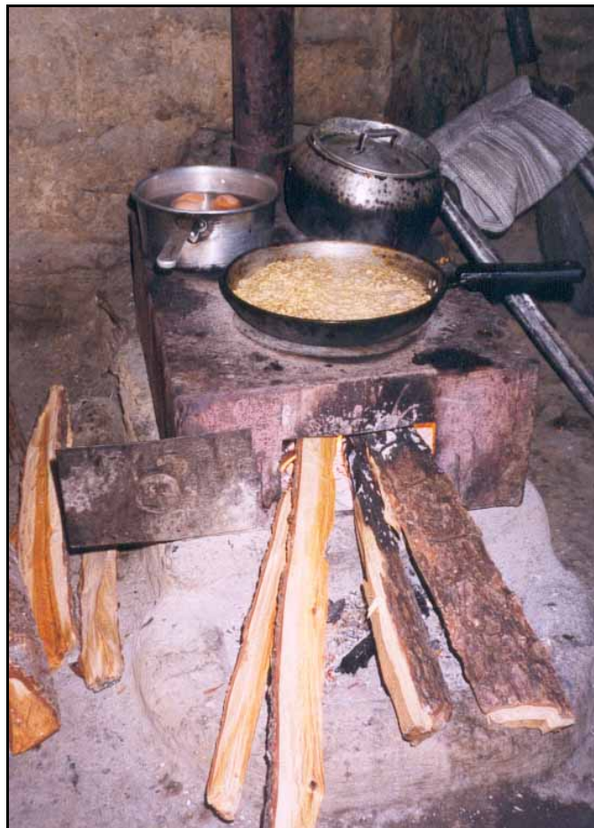
Although many metal stoves have doors, these are never closed. Long sticks of firewood usually lay on the floor in front of the stove. Air intake above the firewood reduces fire temperatures and firewood efficiency.
