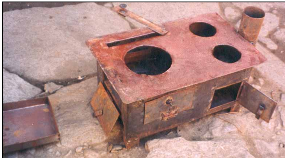
Existing stove type with three doors and roti slot sold without chimney in Dunai for NRs. 5000 (USD 70) 4 . This stove was similar to the first model the KU had introduced in the area.
