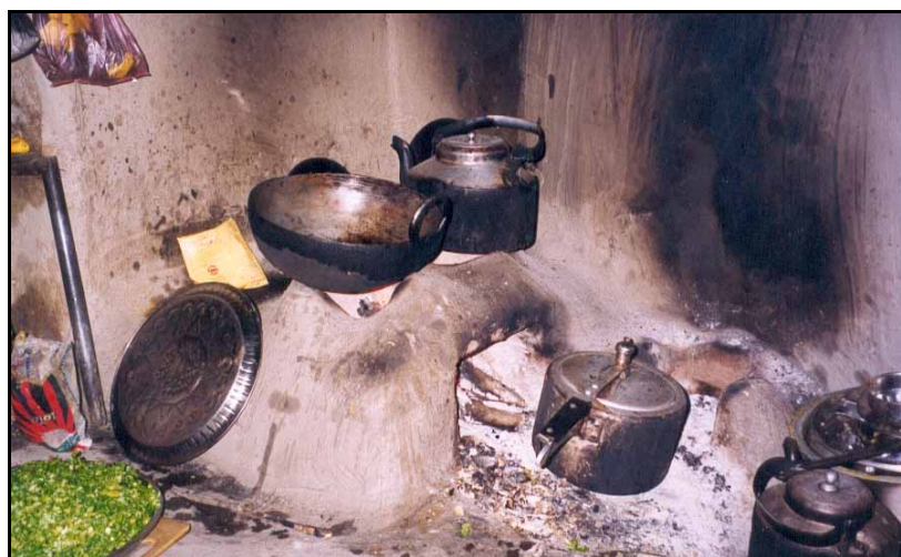
Mud stove for two pots in a restaurant. No chimney. The continuous use of this stove makes it fairly efficient compared to one-meal stoves.
