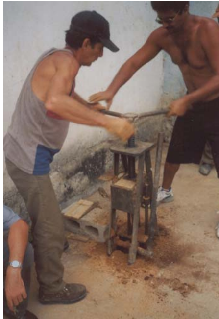
The wet mixture is pressed...
