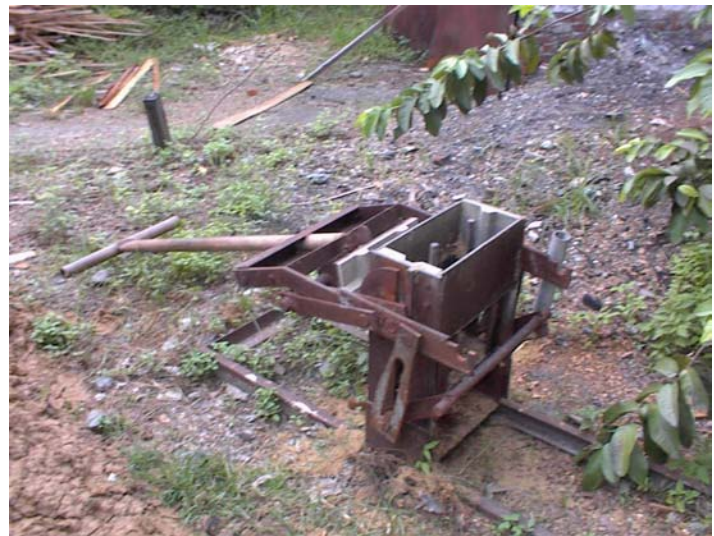
Fig. 4: a) Hand press used for the SFB manufacture, b) Discarded CINVA-RAM press
