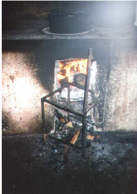
Fig. 3: SFBs initial burning in a cooking stove
