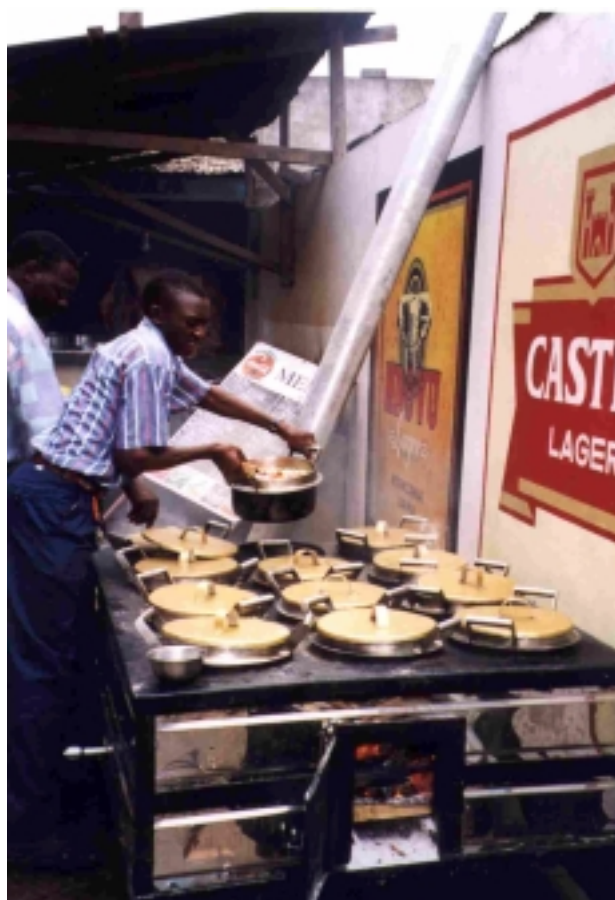
Figure 13: Restaurant now using 12-burner biomass stove with single firebox
