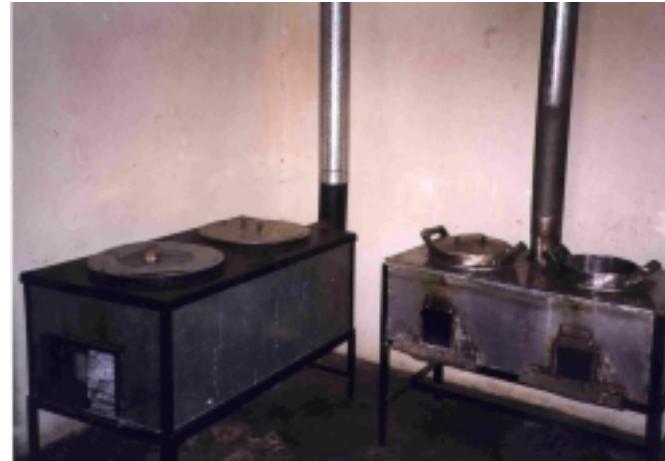
Figure 15: Improved 2 burner stove (left) with original (right), Uganda
