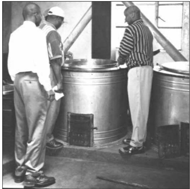
Heavy-duty brick-insulated stainless steel stoves, school kitchen (Kenya).
