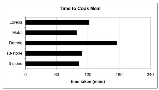
The metal stove, 3-stone fire, shielded 3-stone fire and Lorena are close together at about 100 minutes. Because they are close together, and because the tests change a little every time, especially when cooking food, we cannot be sure that they are not really the same. (see "How can the results be trusted") page 30. The Dembe clearly takes much longer though, the cook must wait an hour more for dinner!
