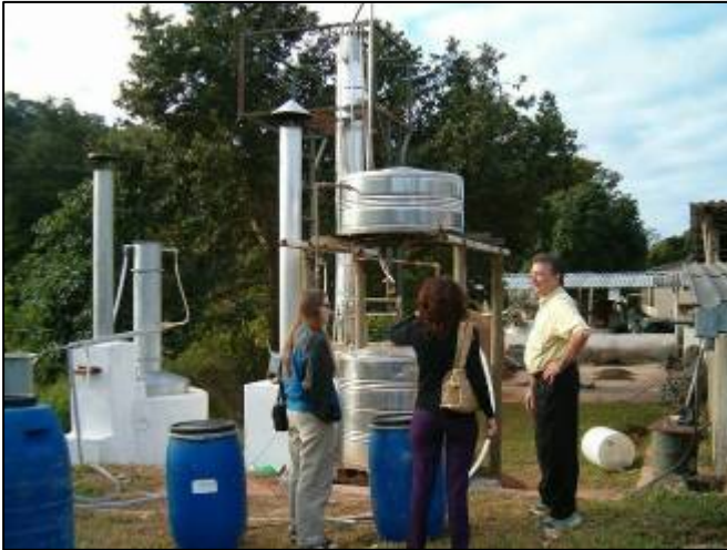
A microdistillery that produces cachaça and ethanol at Viçosa University. Professor Juarez de Souza is very interested in Project Gaia, and has agreed to explore a possible partnership between the university and Project Gaia to carry out an additional study on the concept of local cooperatives producing ethanol for household energy use.
