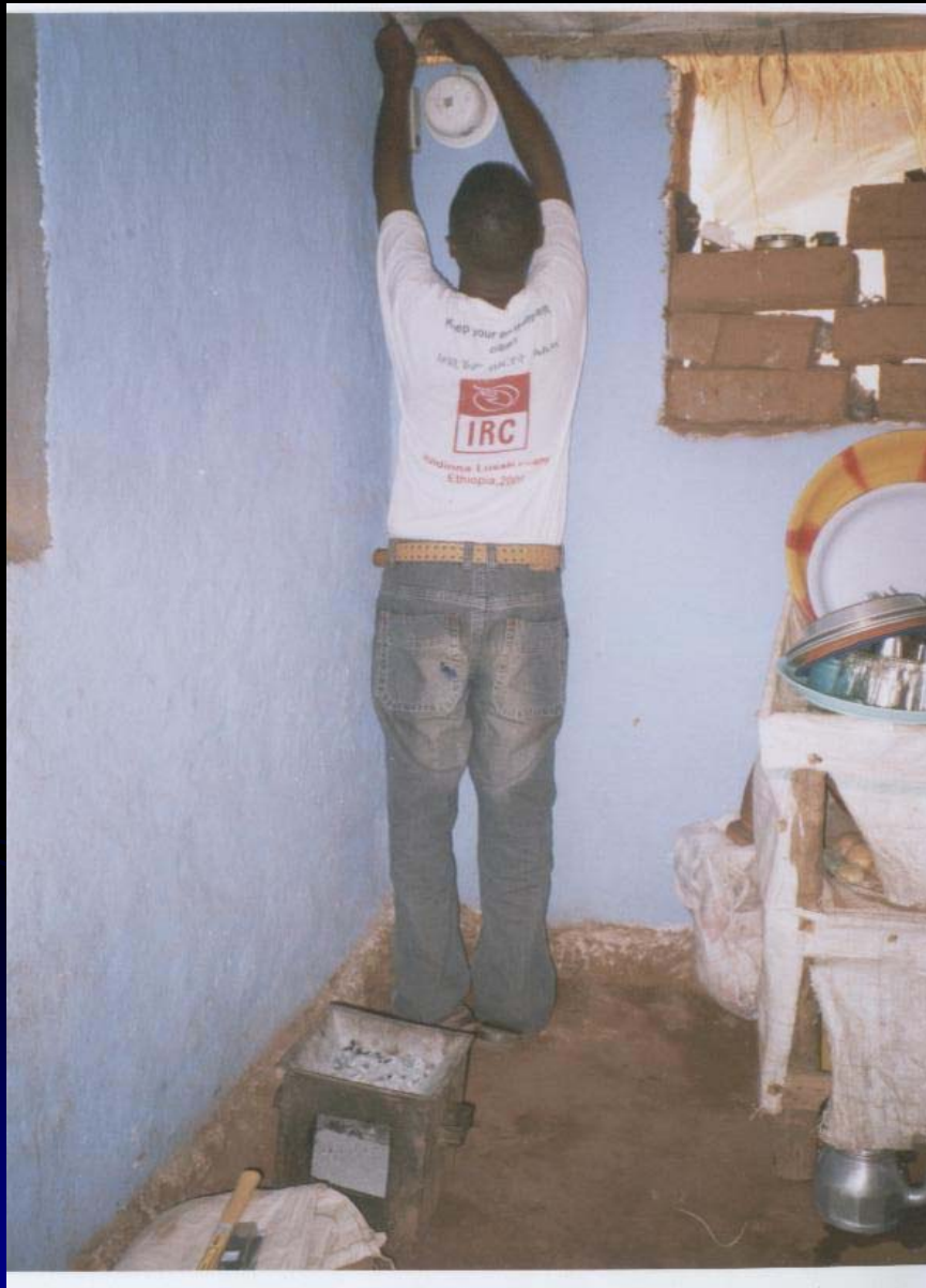
Shimelba Refugee Camp (UNHCR) Indoor Air Pollution Monitoring Surveyor placing IAP measuring instruments
