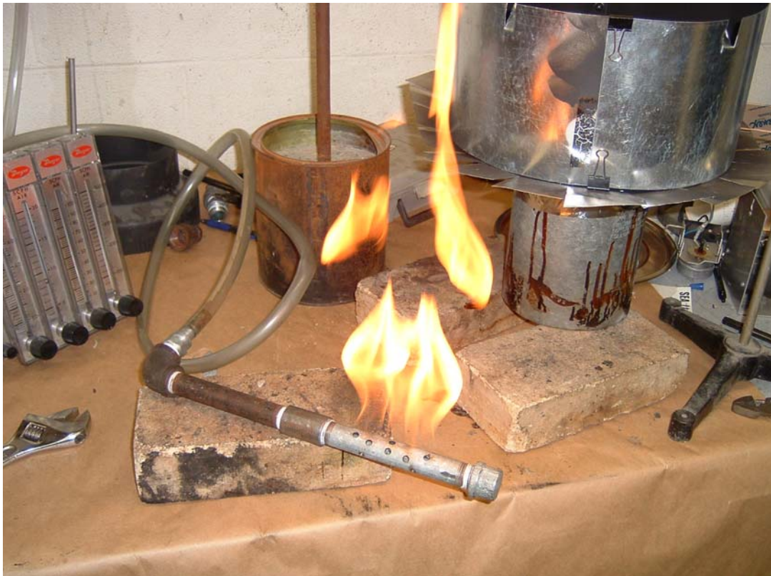
Figure 3: The simulated wood flame. The flame has a “tongued” appearance due to the camera flash.
