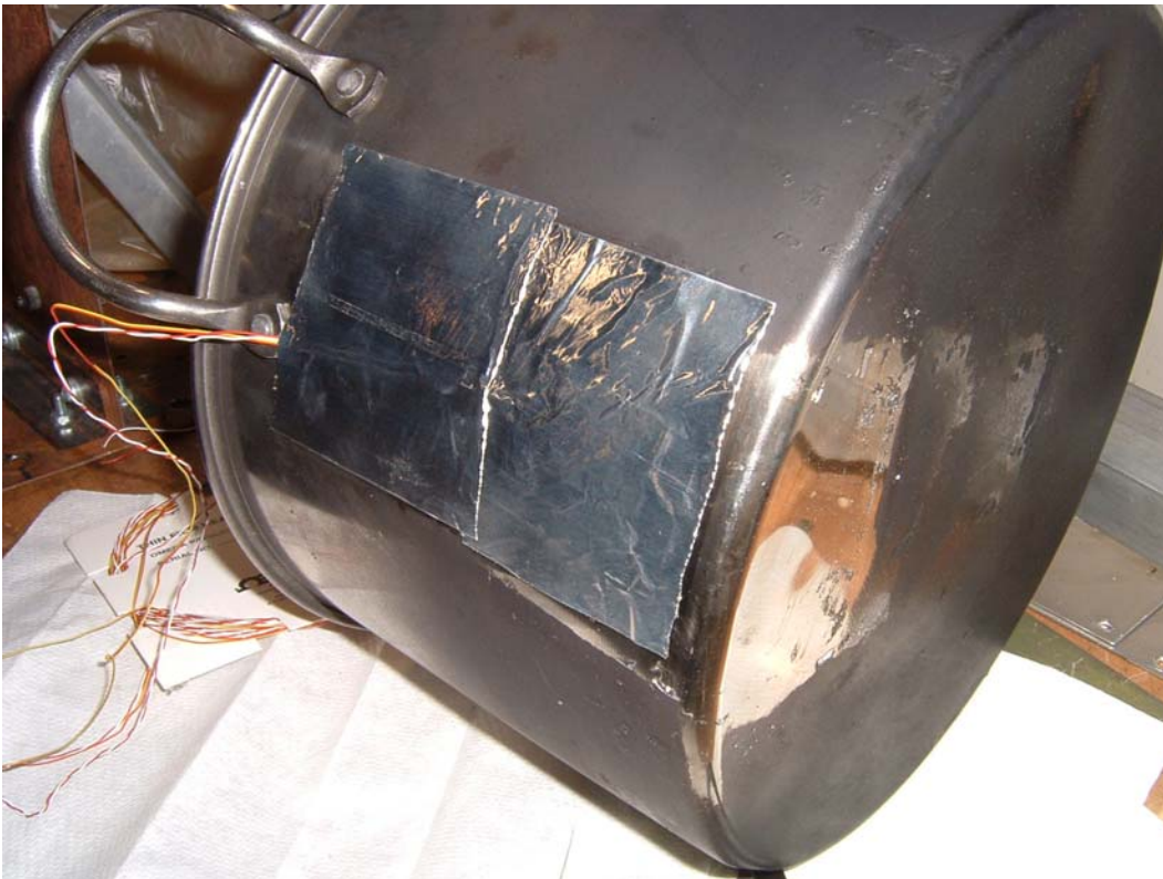
Figure 2: The heat flux sensor after being covered by reflective tape.
