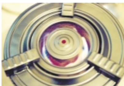
Figure 2: Top view of a stove in operation. Note red heat of inner element and blue "jets" at 8 o'clock
