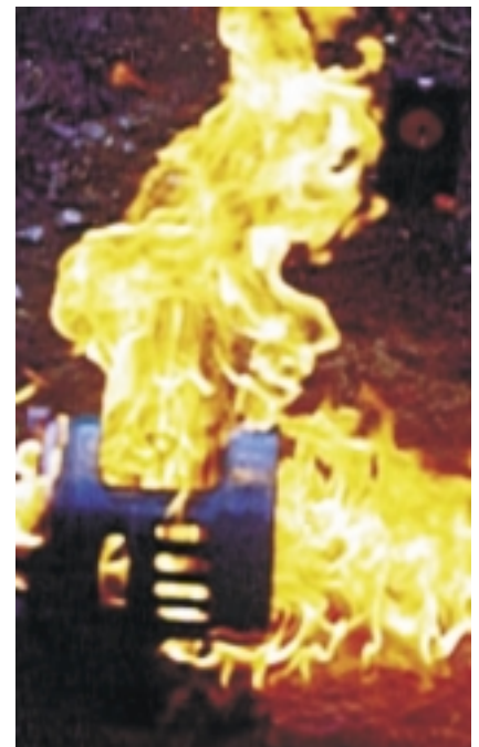
Figure 5: Five seconds after knocking stove over
