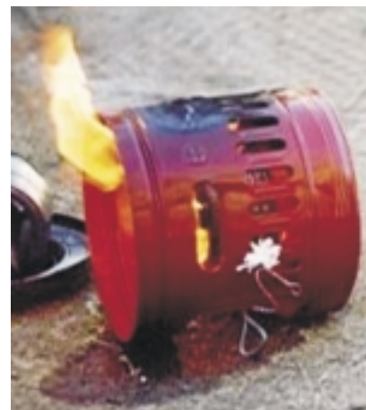
Figure 7: Stove containing cold paraffin. 50 seconds after knocking stove over.
