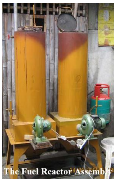
The Fuel Reactor Assembly
