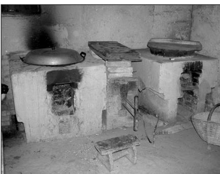
Figure 2 Unvented stove with bellows (photo: Kirk Smith)
