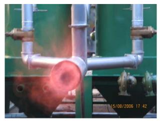
velocity of the reactors averages to 148.5 kg/hr-m<sup>2</sup> and 5.4 cm/sec, respectively. The percentage amount of char produced is 35%. One person is needed to attend in loading and unloading of fuel from the reactor. Actual tests showed that the gasifier can continuously supply the required heat that is needed by a 6-ton
