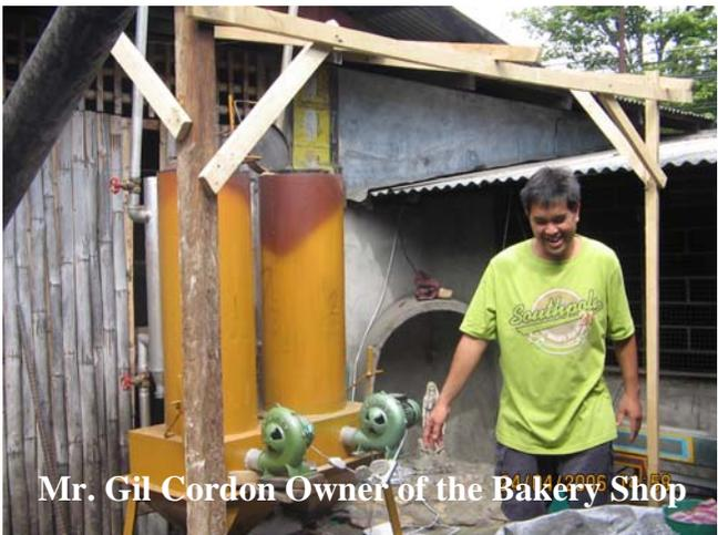
The rice husk gas burner featured in this article is owned by Mr. Gil Cordon, a baker from Jaro, Iloilo City. According to him, he uses LPG fuel for 10 minutes to start-up the oven and after that shifts to the rice husk gas burner until operation is done. He also uses LPG fuel as back up in case of power failure. Both ovens are simultaneously used when baking “Pande leche,” “Pande sal,” and other similar bread. When baking “Mamon” and “Hopia” either one or two ovens LPG back-up is used.
