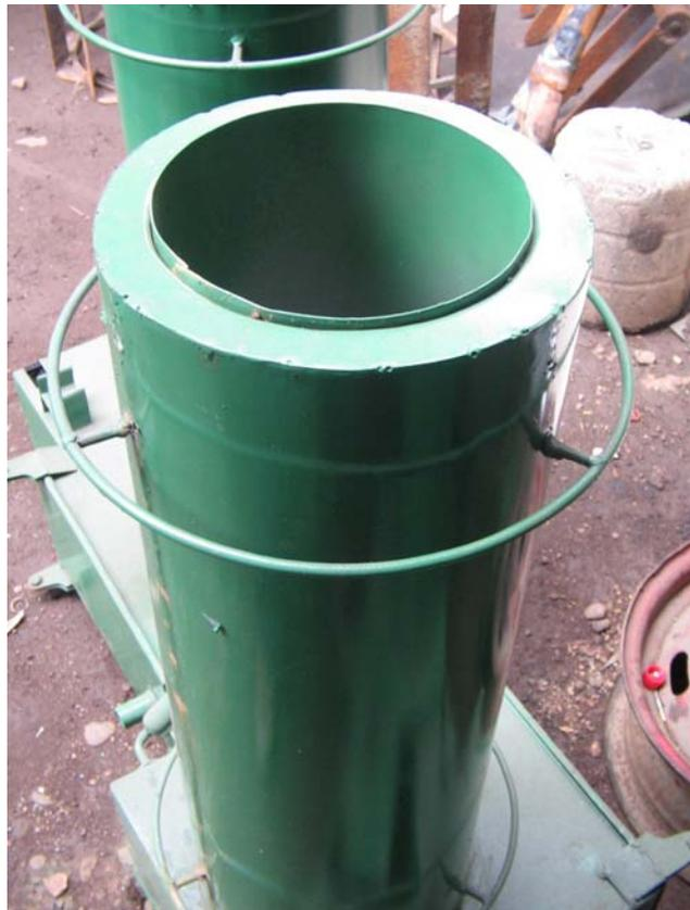
Figure 6. The Gasifier Stove Reactor.
