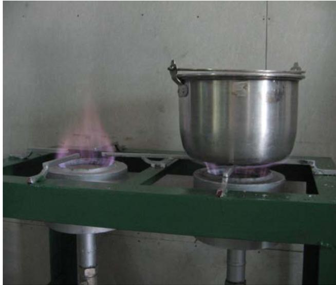
Figure 81. The Bluish Flame Produced in the Stove.
