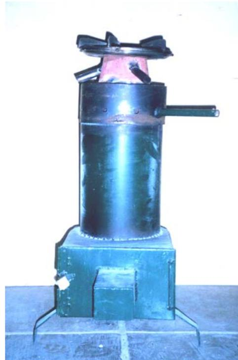
Figure 23. The CPU IDD/T-LUD Wood Gas Stove.
