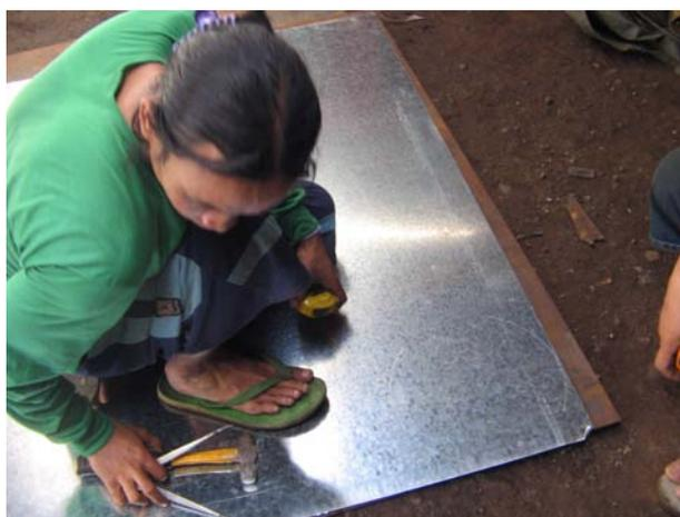
Figure 54. Layouting of Stove Parts.
