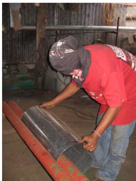
Figure 56. Forming Cylinders on Pipe Bender.
