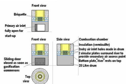
Figure. 33. The Holey Briquette Gasifier Stove.
