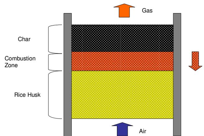
Figure 36 B. Inverted DownDraft Type Gasifier is Top-Lit with UpDraft
