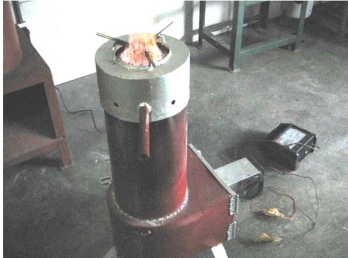
Figure 20. The CPU Proto-Type IDD/T-LUD Rice Husk Gas Stove Model 2.
