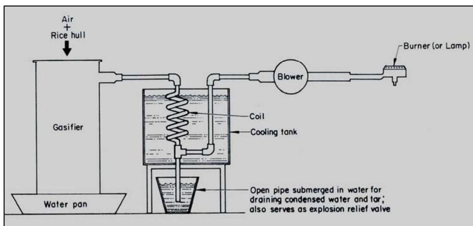
Figure 16. Schematic Drawing of the DA-IRRI Rice Husk Gasifier.
