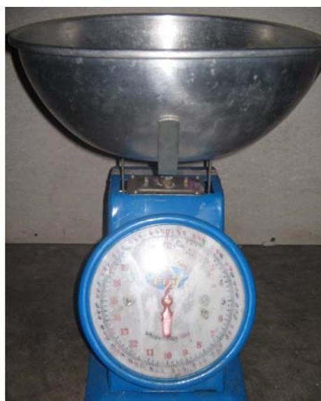
Figure 65. The Spring-Scale Balance
