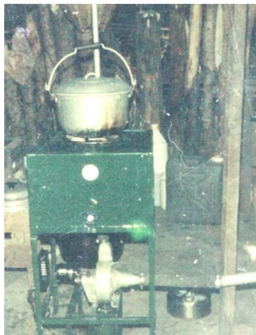
Figure 17. The CPU Single-Burner Rice Husk Stove.
