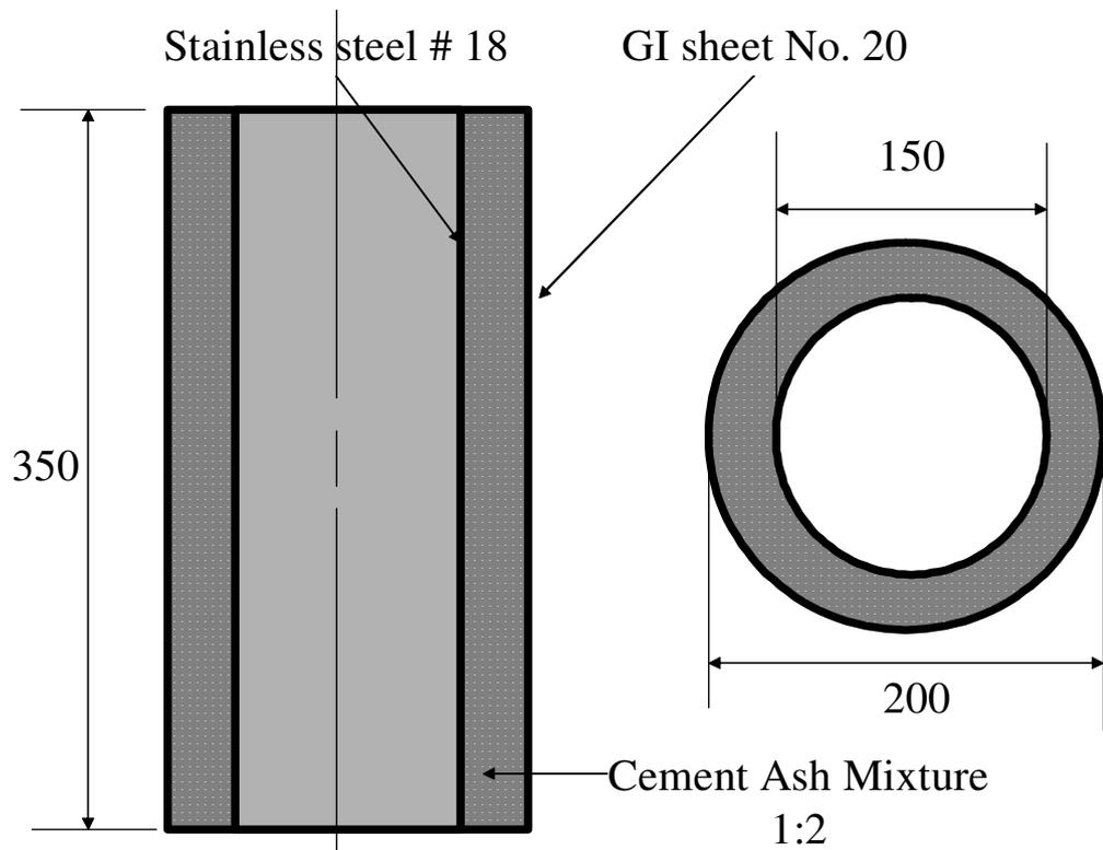
Detail of Fuel Cylinder Assembly
