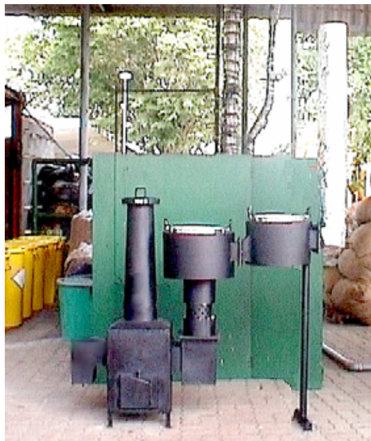
Figure 2.17: Fully assembled gasifier stove IGS2, with pot support
