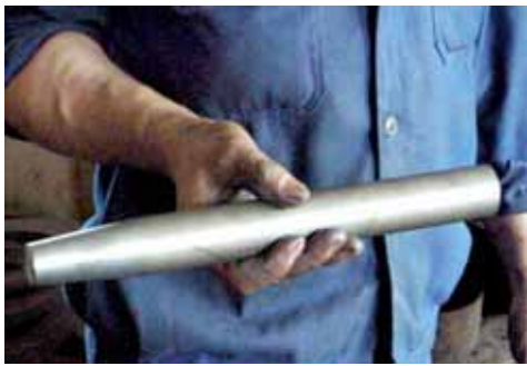
(i). Screw shaft turned in a lathe
