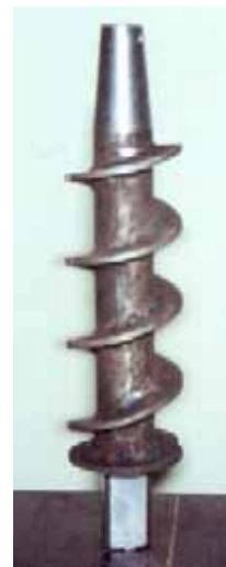
(iv). Completed screw, ready for installation
