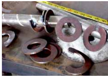
(ii). Washers as screw threads
