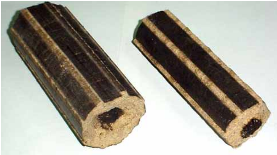
Figure 7.1: The 71 mm and 55 mm briquettes produced with the above briquetting machines
