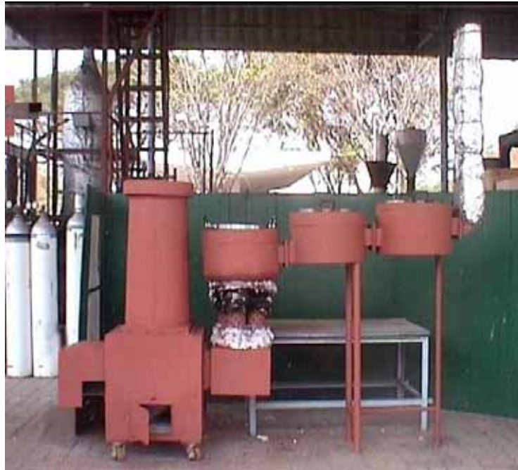
Figure 3.16: Fully assembled gasifier stove CGS3 with three-pot support.
