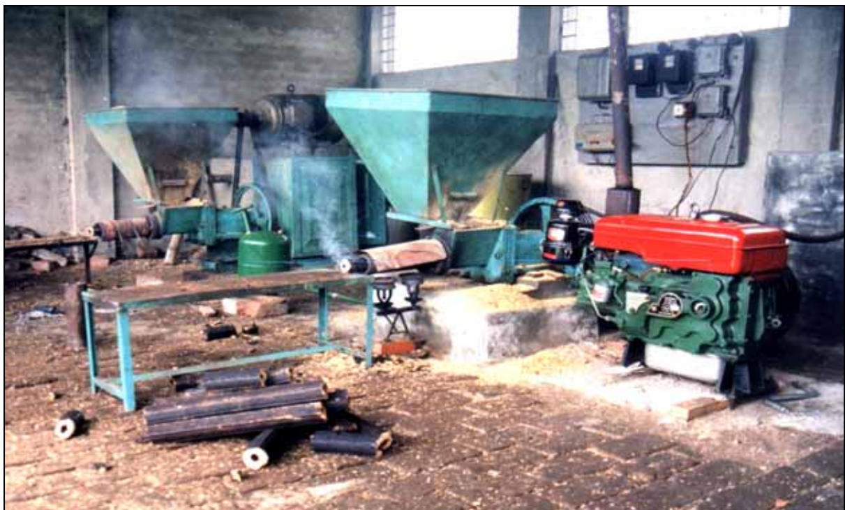
Improved briquetting machine with diesel engine, Bangladesh
