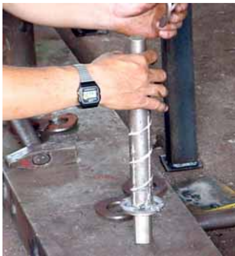
(iii). Inserting washers over the screw shaft
