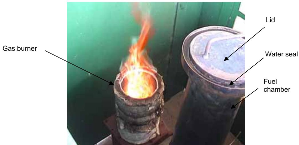
Figure 2.16: Combustion in the gas burner
