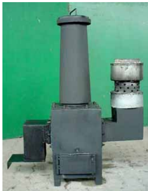
Figure 4.14: Fully assembled Domestic Gasifier Stove without pot support
