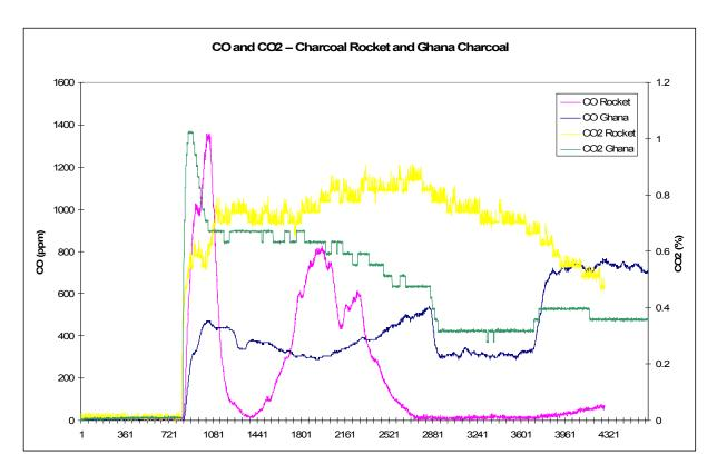
It can be seen that even though the CO level for the rocket drops below 10 ppm, the CO2 level remains high suggesting a high firepower continues. The Ghana charcoal stove has a lower level of CO2 with a considerably higher level of CO.
