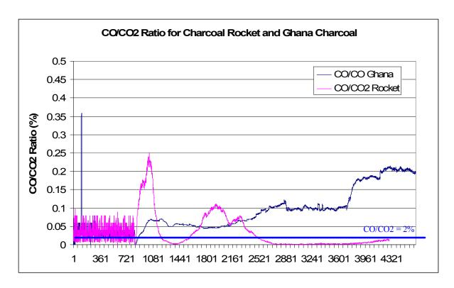
Higher ratios mean the stove was making more CO and less CO2. Perfectly efficient combustion would produce all CO2 and no CO because the CO is combusted and changed into CO2.
