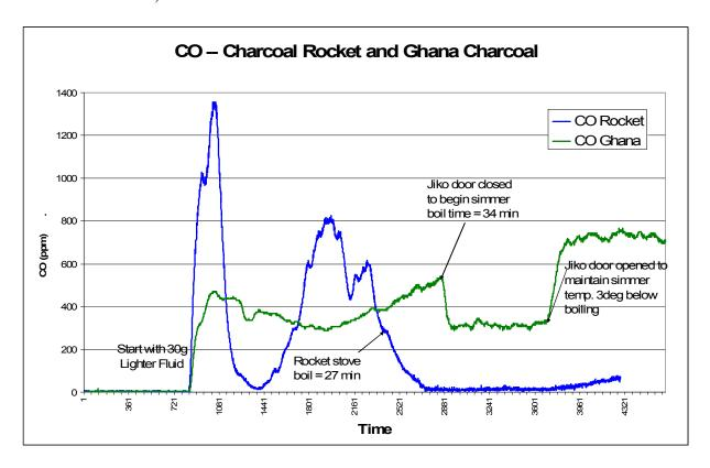
As previously reported, emissions of CO in the Jiko-type stove are reduced when the door is closed. Opening the door to increase firepower, in an effort to maintain simmering temperatures, increased emissions. The rocket stove maintained a full boil during the simmering period.
