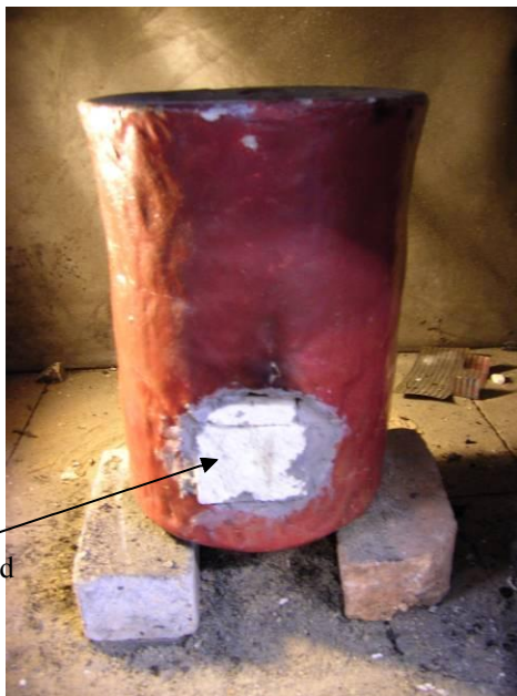
Grate under chimney to hold charcoal
