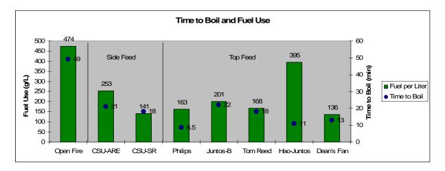
Results of testing under the emissions hood, one abbreviated water boiling test per stove:
