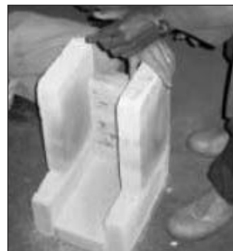
Figure 4 Combustion chamber in rocket stove being made (photo: Peter Scott)
