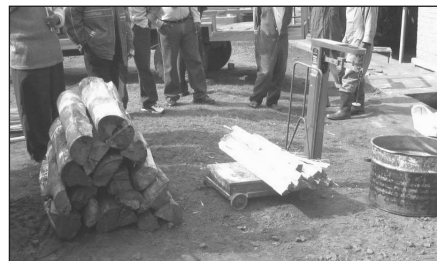
Figure 2 Quantities of fuel used by open fire and rocket stove to cook equal quantities of food (photo: Peter Scott)
