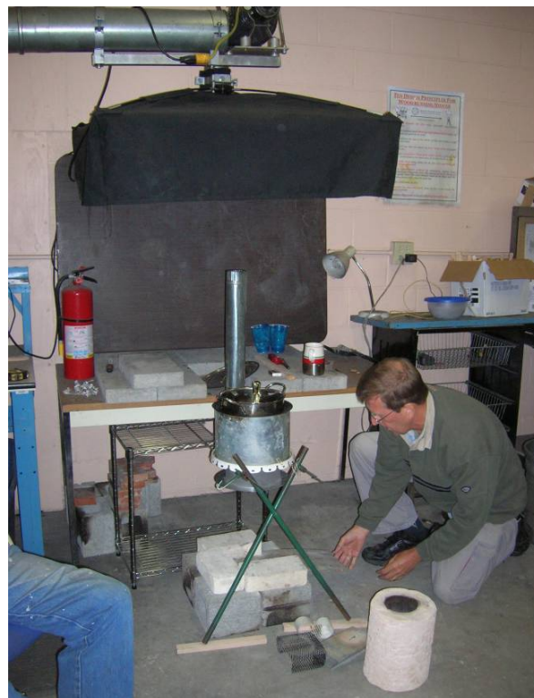
One of Paul Anderson's gasifier stove setups, with interchangeable ceramic and fan-assisted combustion chambers.
