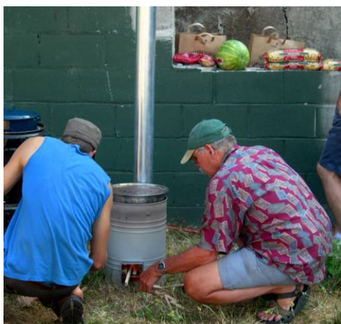
Damon's 10L pot sunken pot Rocket stove with chimney works with both pot and griddle. An internal skirt makes this stove fuel efficient.
