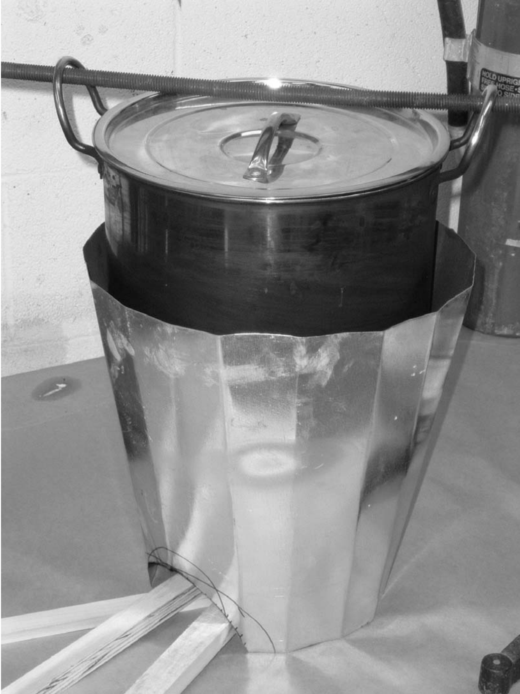
Fig. 8.2: The prototype tapered-sided skirted campfire stove. (Yes, it looks like a wastebasket!)
