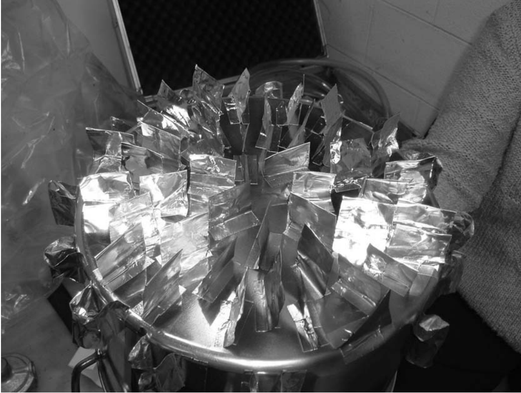
Fig. 7.1: The prototype finned pot used with the Fischer burner. The fins protrude about 25 mm from the bottom of the pot.
